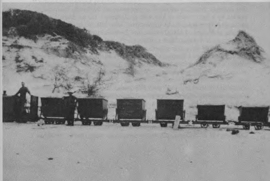
Illustr. 12. Hauling black sand from beach by trucks and diesel locomotive, Yamba, circa 1937. (By courtesy late W. H. Derrick)
