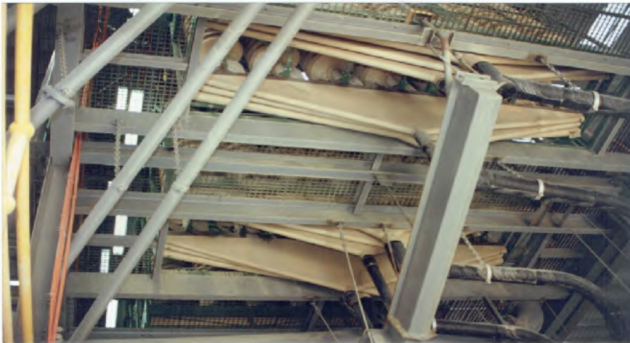
Reichert Spirals in Tantalum circuit at Gwalia Consolidated, Greenbushes, WA
