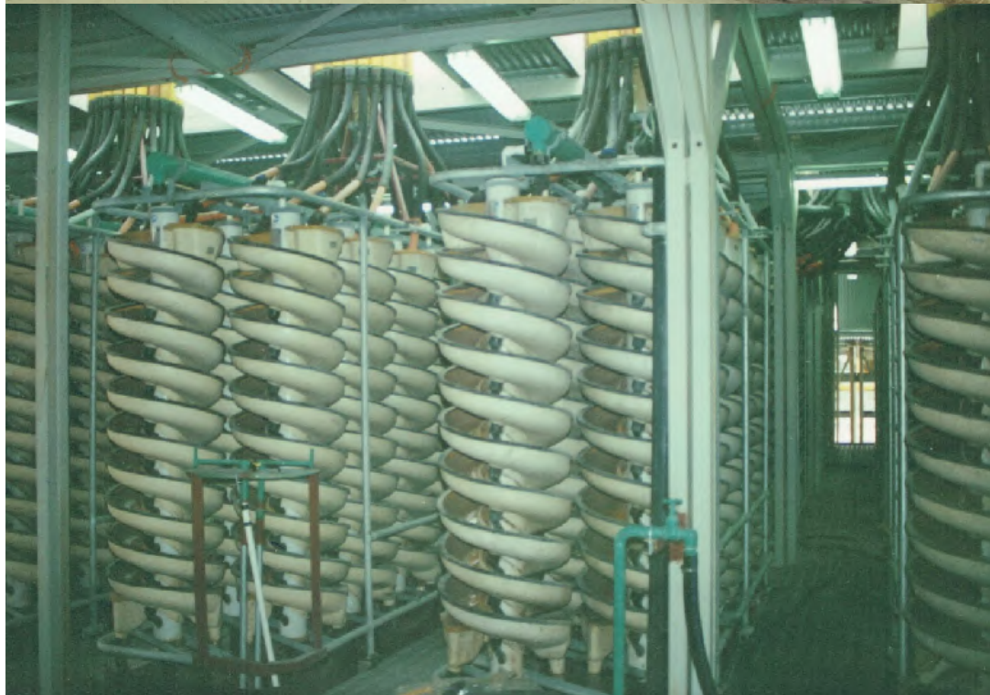
900 tph Minerals Sands Spiral Plant for Cable Sands at Jangardup, WA
