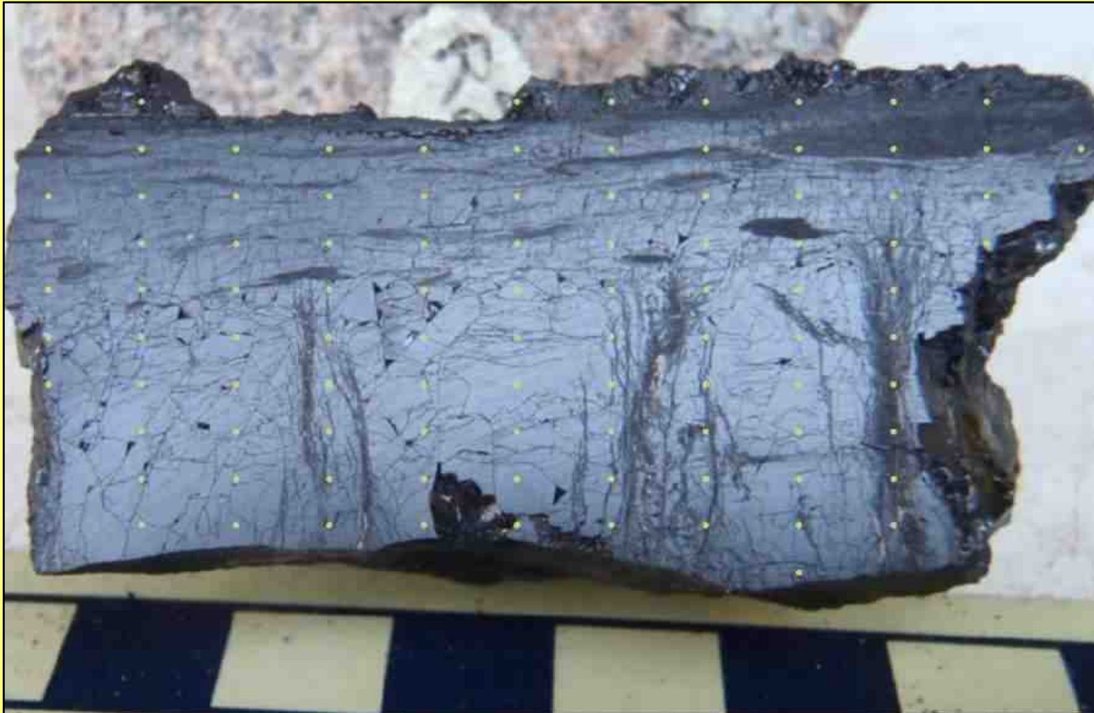
Figure 9: Polished section of HQ (61 mm) core showing structure. Vertical dots at 2.5 mm spacing, horizontal dots at 5 mm spacing
