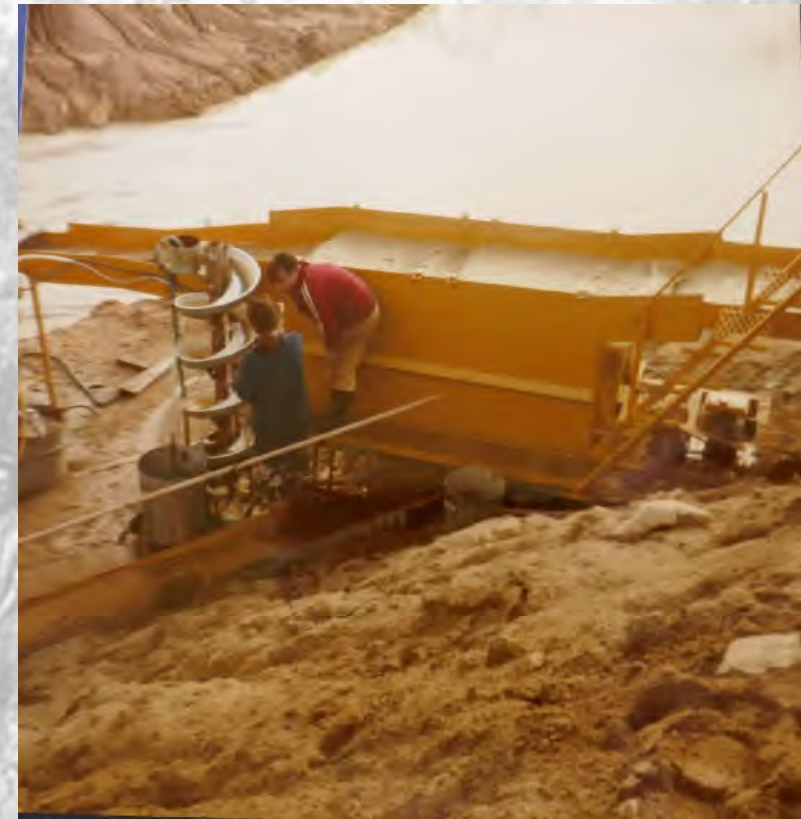
Fat Cat Mine Arbouin Gully at Sugarloaf- Concentrating plant jig and spirals Circa 1993
