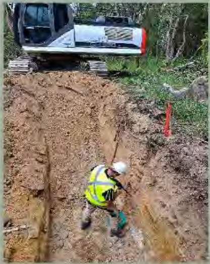
Channel sampling in alluvial bulk pits
